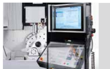
E. Control Panel Ergonomic operation panel with adjustable angle.
