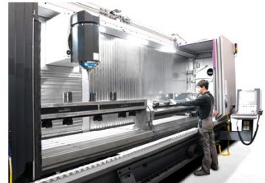
Tilting head. Flat fixed table where rotary tables can be bolted
